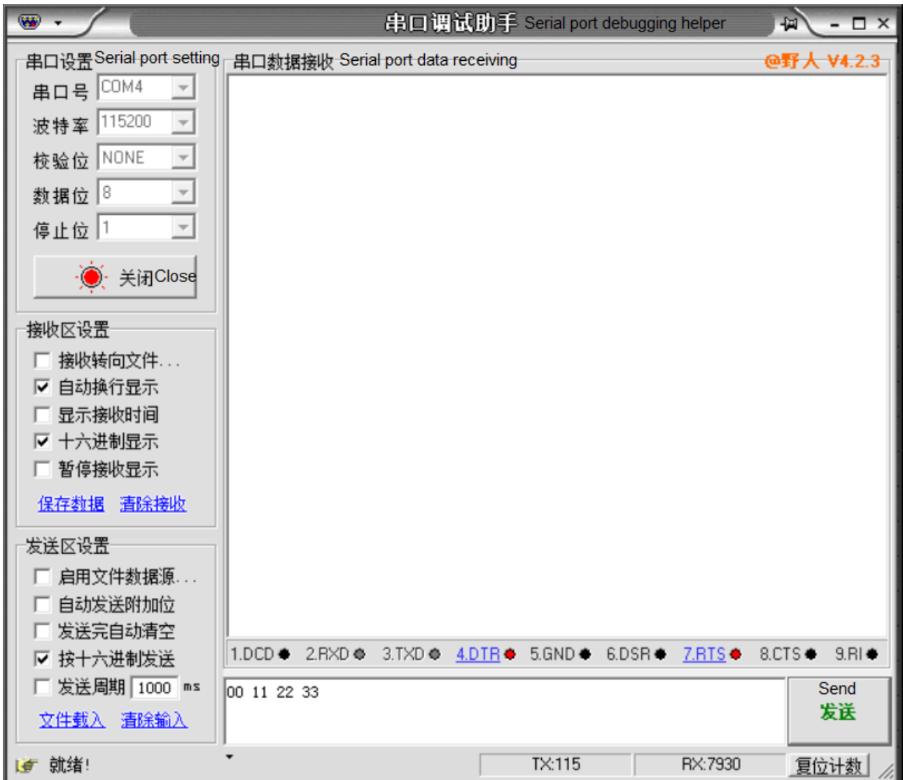
Figure 16.7: Sending 4 data using the serial port tool
