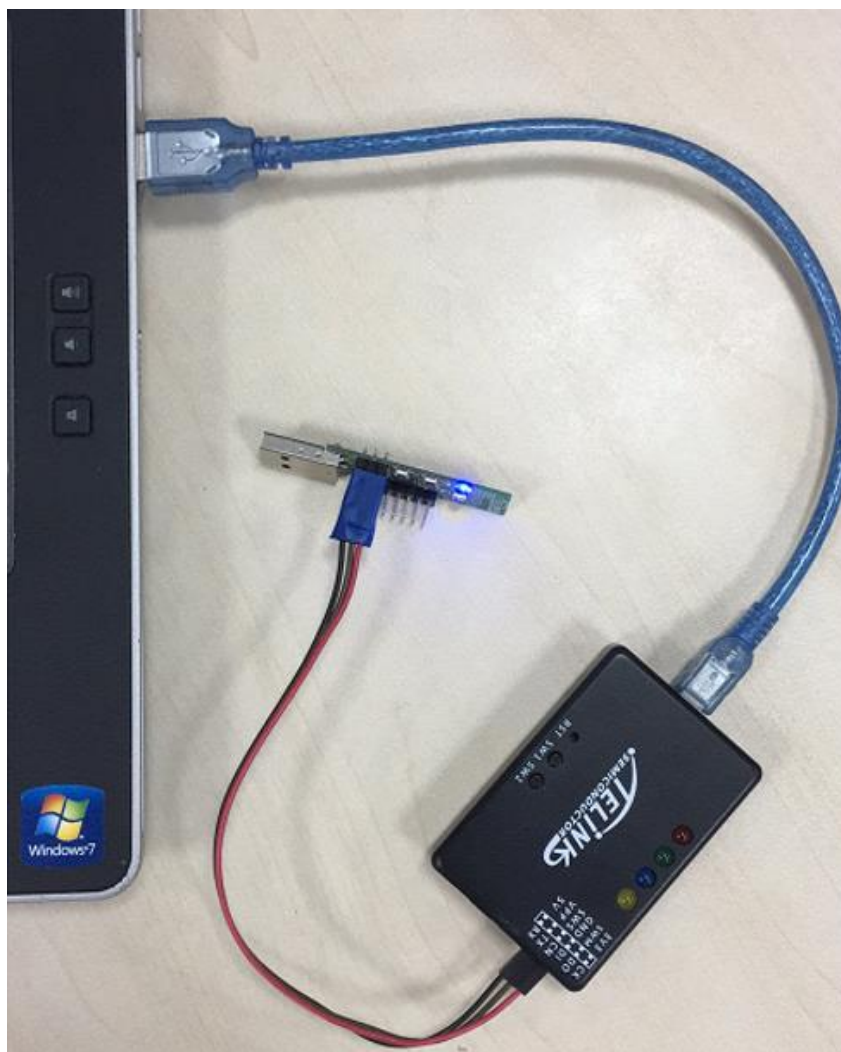
Figure 6 Connection chart for target board, burning EVK and PC
