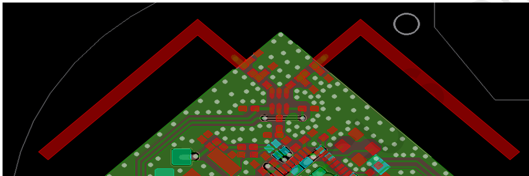
Figure 3 Good design example: dual antenna with vertical placement
