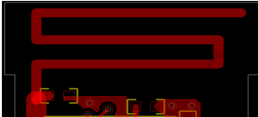
Figure 6 Bad design example: route exposed to antenna
