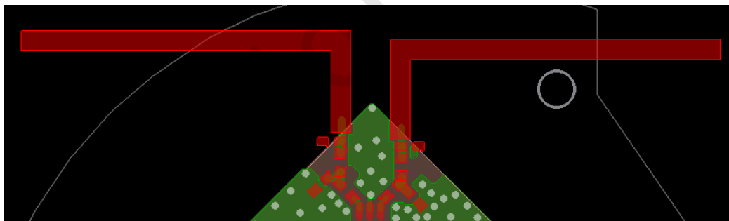
Figure 4 Bad design example: dual antenna with non-vertical placement
