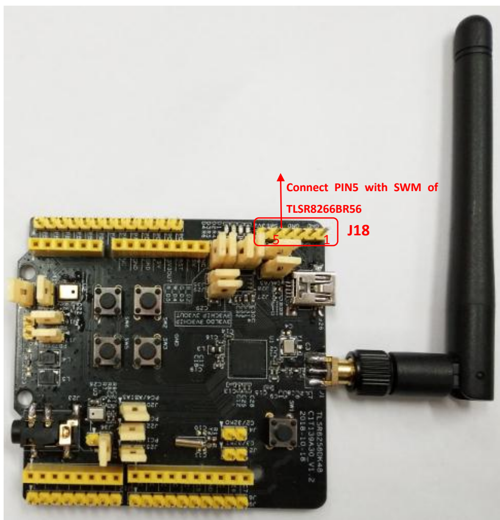
Figure 8 Connection chart to download firmware
