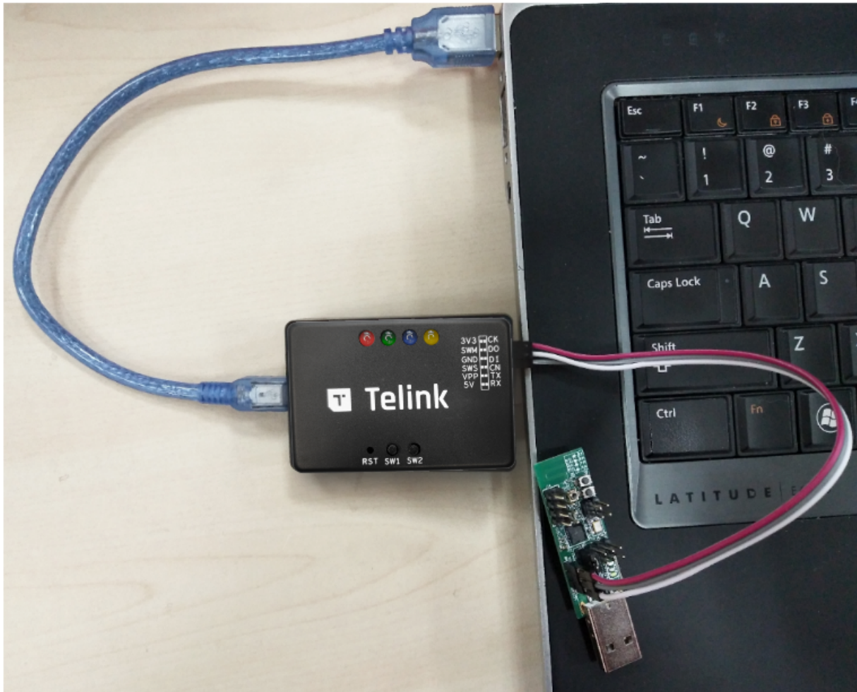
Figure 2.4: Connect target board with "Burning EVK" via Swire
