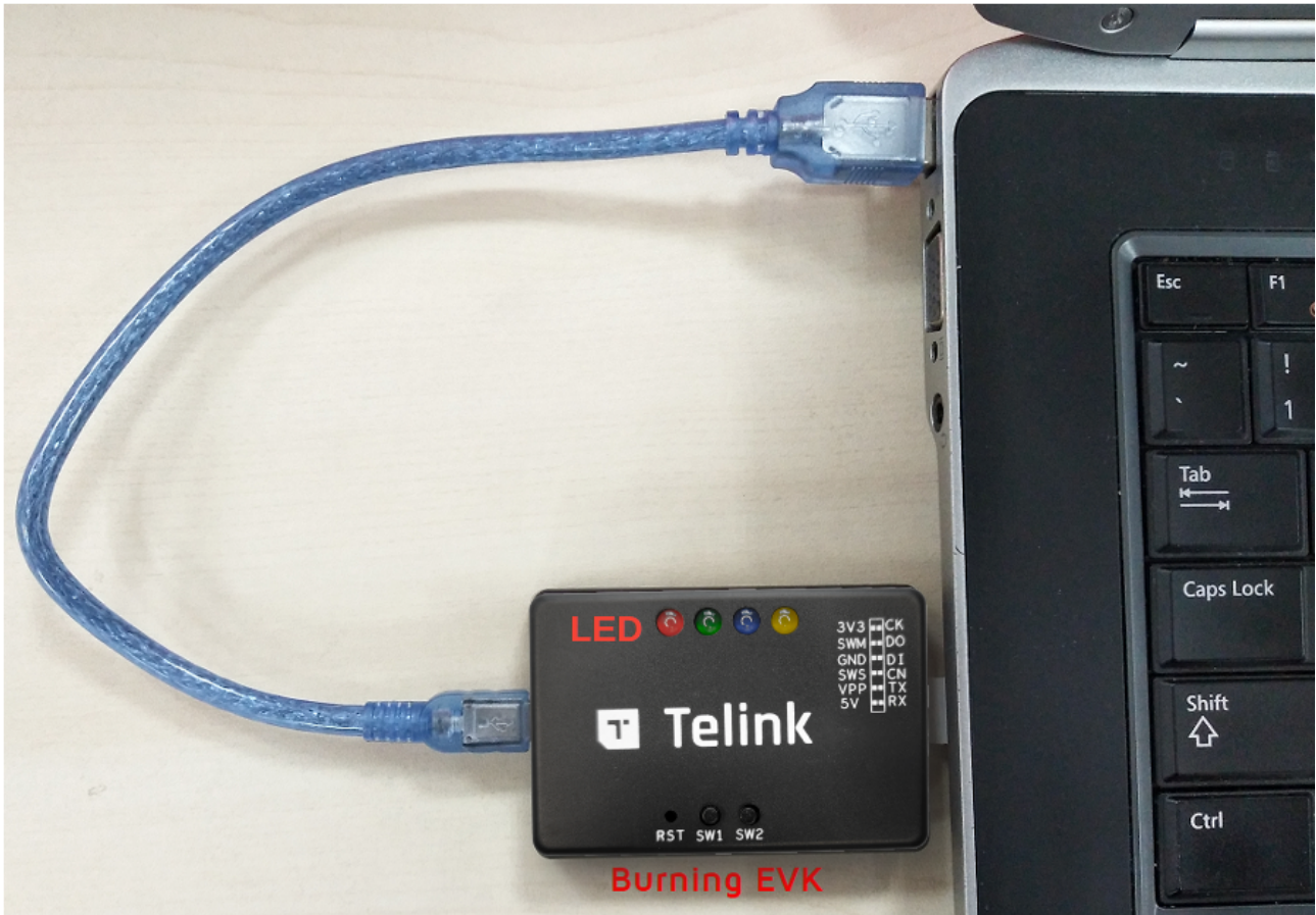
Figure 2.2: Connect "Burning EVK" with PC
