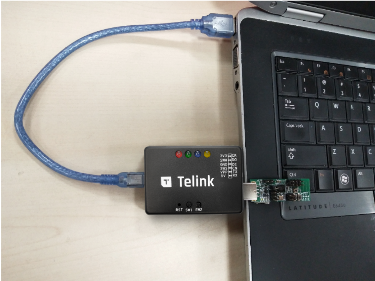
Figure 2.3: Connect target board with "Burning EVK" via USB
