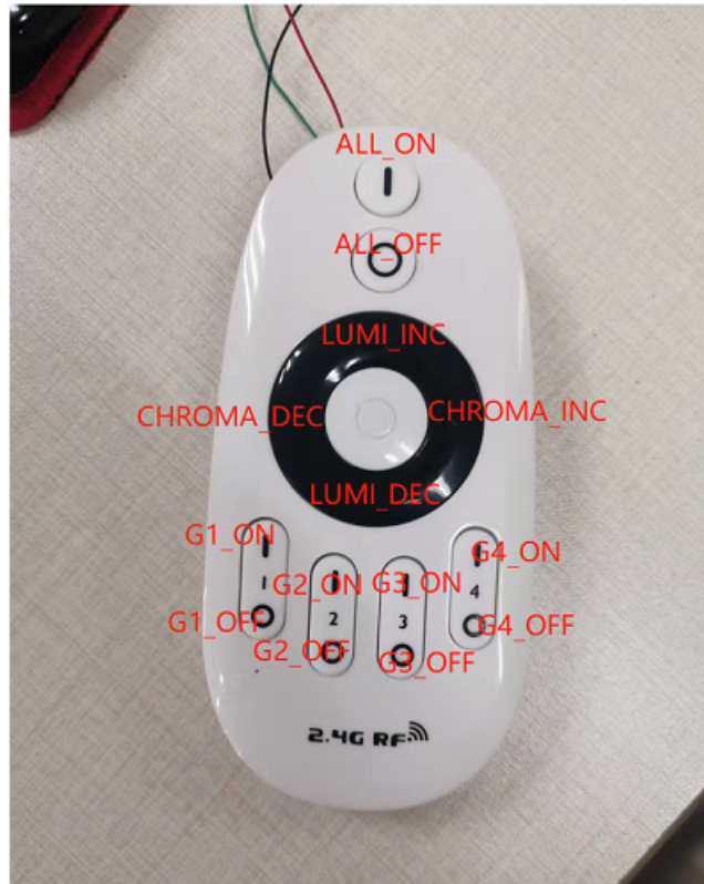
Figure 4.1: "REMOTE&LIGHT and REMOTE_BEACON&LIGHT_BEACON keys introduction"
