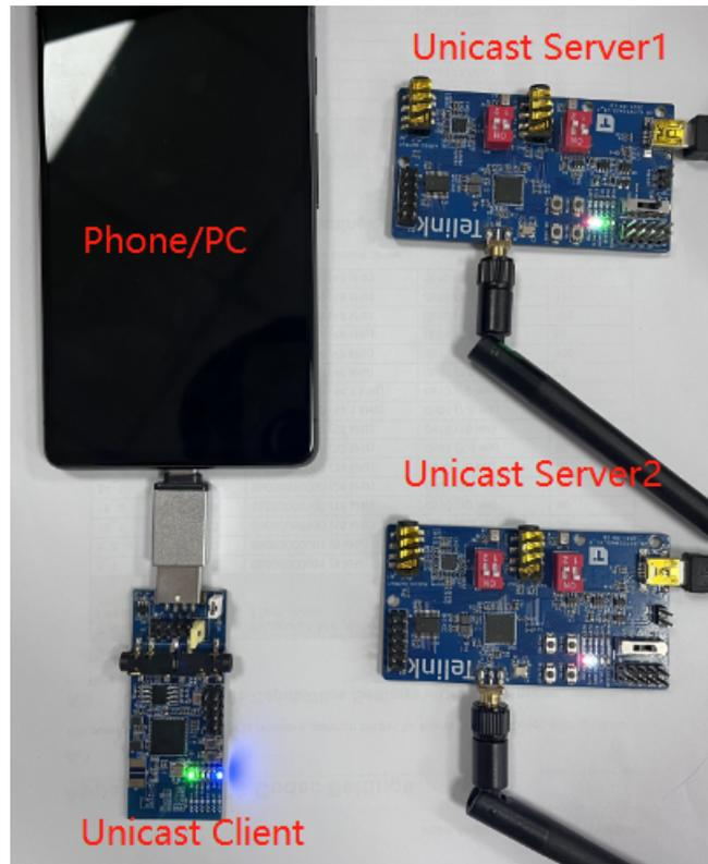
**Figure 2.3:** Unicast scenario 1 environment setup
