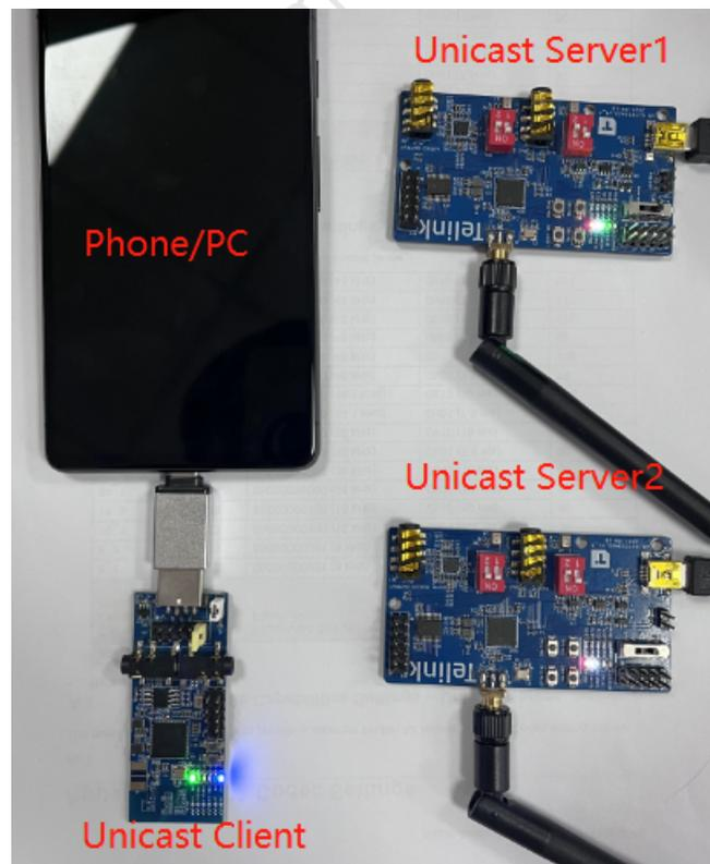
**Figure 2.6:** Unicast scenario 2 environment setup
