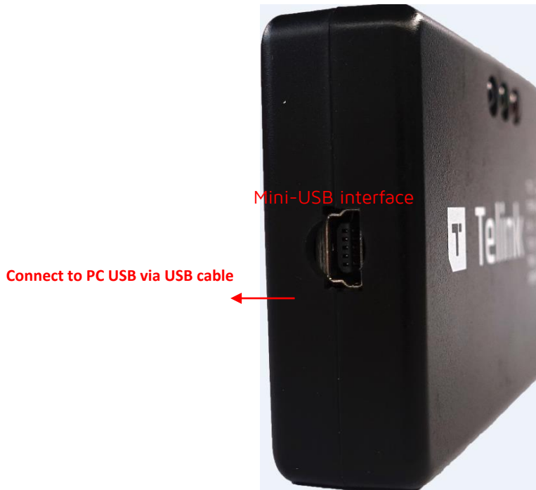
Figure 2-1 Connection chart to supply power for TLSR9_DEV_KEY
