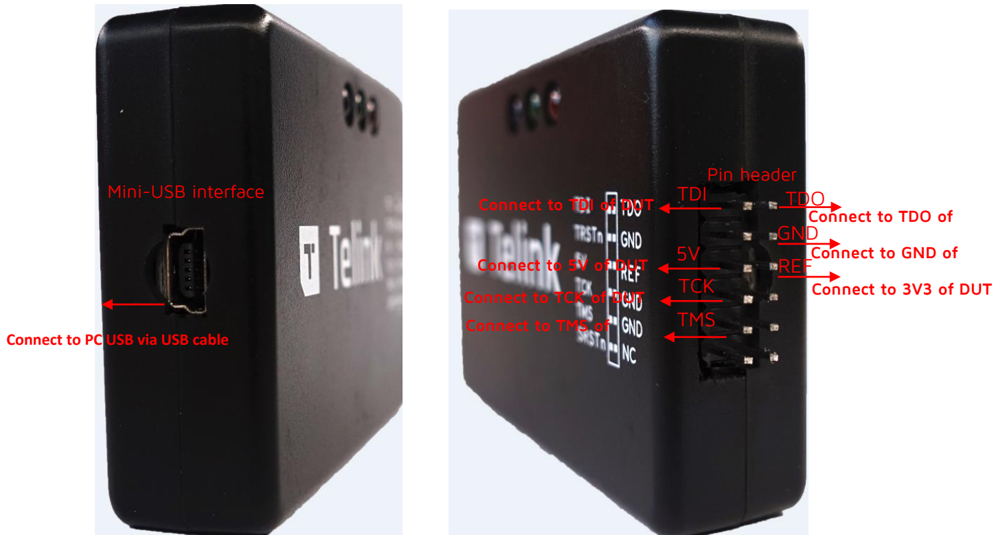
Figure 2-2 Connection chart 1 to download FW into DUT via TLSR9_DEV_KEY
