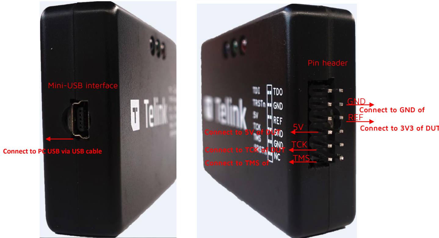
Figure 2-3 Connection chart 2 to download FW into DUT via TLSR9_DEV_KEY
