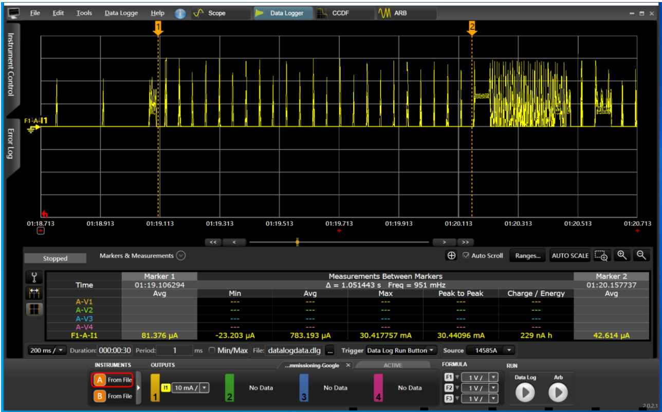
Figure 10.4: BLE connection interval average current @ 45ms
