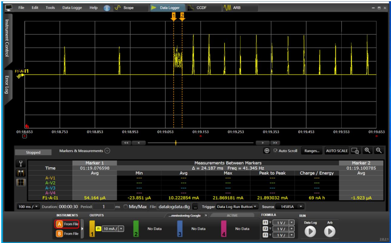
Figure 10.6: BLE connection request current cost
