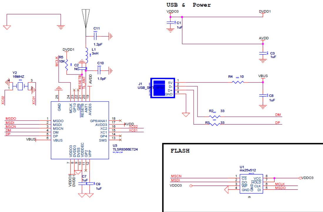
Figure 12- 3      Schematic for the TLSR8366ET24
