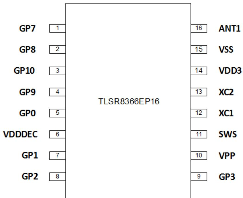
Figure 1- 7 Pin assignment for the TLSR8366EP16
