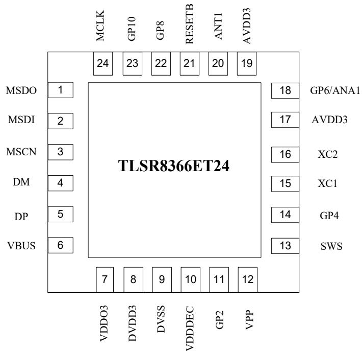
Figure 1- 6 Pin assignment for the TLSR8366ET24
