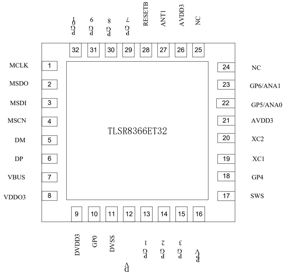
Figure 1- 5 Pin assignment for the TLSR8366ET32
