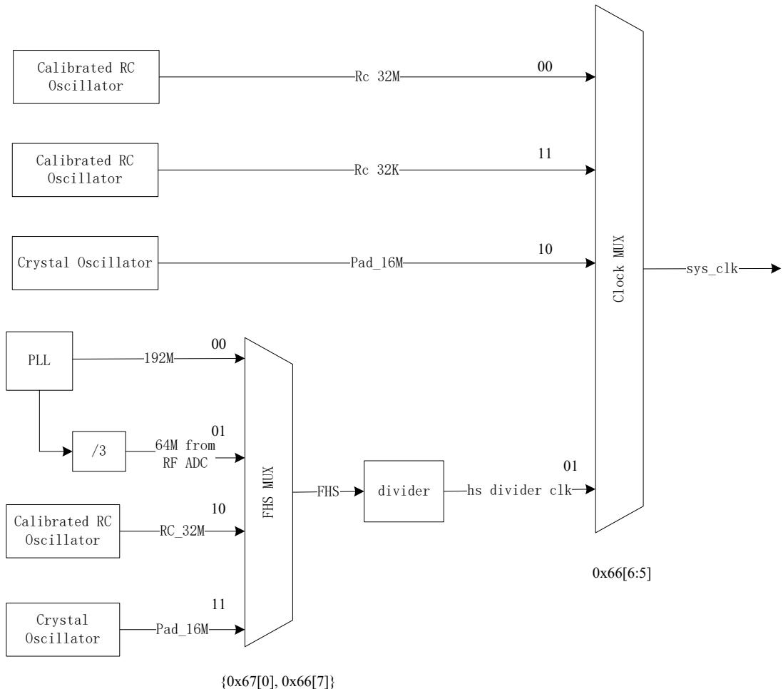
Figure 5- 1 Block diagram of system clock
