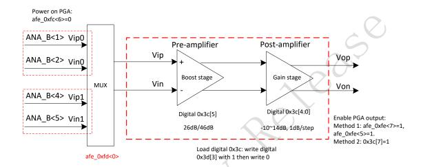
Figure 11-1 Block diagram of PGA
