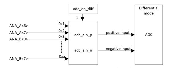
Figure 10- 1 Block diagram of ADC
