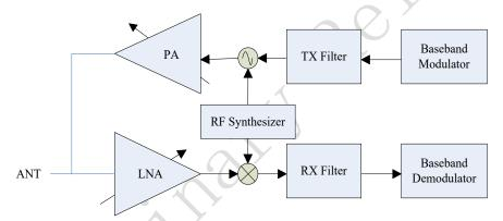
Figure 3-1 Block diagram of RF transceiver
