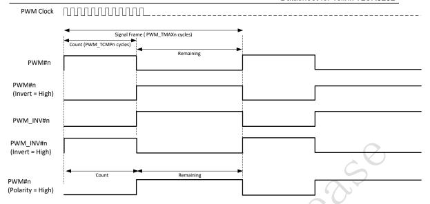
Figure 8-2 PWM output waveform chart
