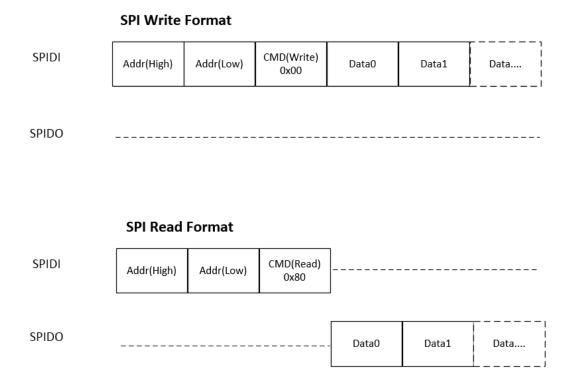
Figure 7-8 SPI write/read command format
