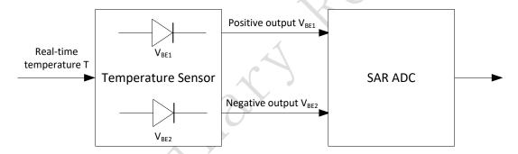
Figure 12-1 Block diagram of temperature sensor
