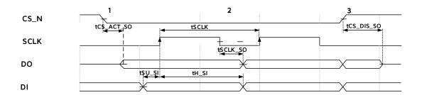
Figure 15-3 SPI Timing Diagram, Slave Mode
