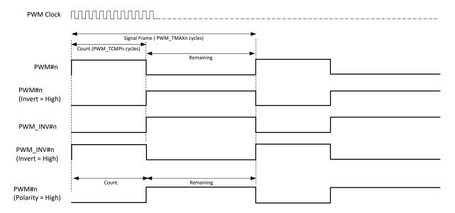
Figure 8-2 PWM output waveform chart
