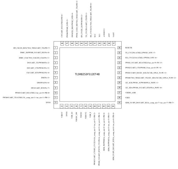
Figure 1-4 Pin assignment for TLSR8253F512ET48
