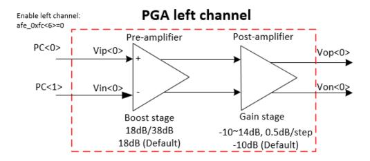
Fix input channels: afe\_0xfd=0x55
