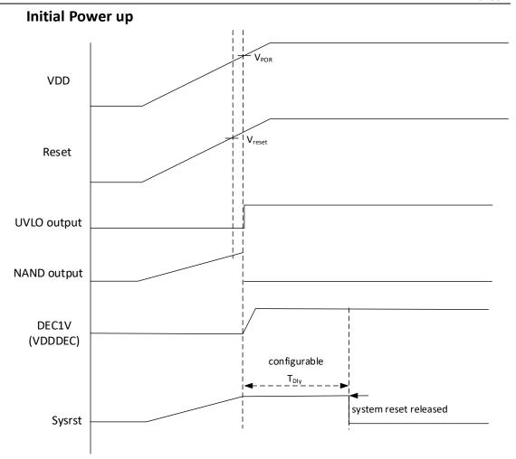
Figure 2-4 Initial Power-up sequence
