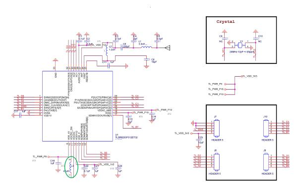
Figure 16-2 Schematic for TLSR8253F512ET32
