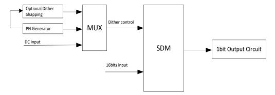
Figure 9- 6 Block diagram of SDM
