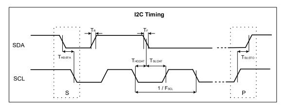
Figure 15-4 I2C Timing Diagram
