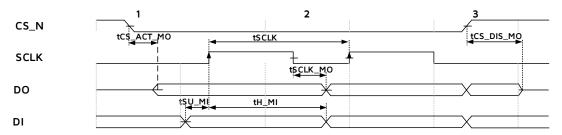
Figure 16-2 SPI Timing Diagram, Master Mode
