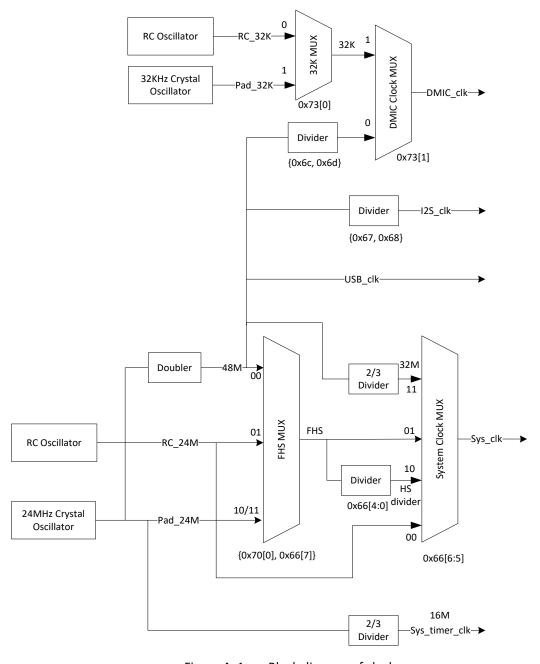
Figure 4- 1 Block diagram of clock
