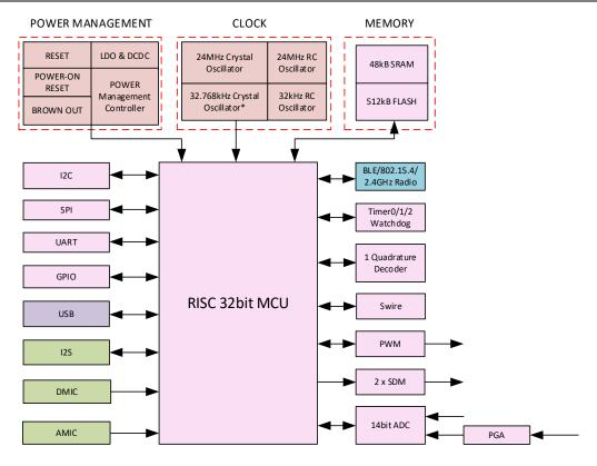
Figure 1-1 Block diagram of the system
