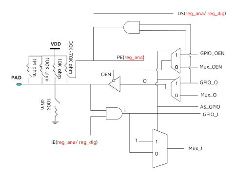
Figure 7-1 GPIO logic diagram
