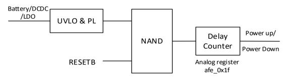
Figure 2-3 Control logic for power up/down
