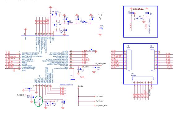
Figure 16-1 Schematic for TLSR8253F512ET48
