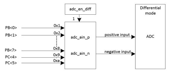
Figure 11-1 Block diagram of ADC
