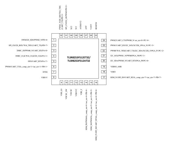
Figure 1-5 Pin assignment for TLSR8253F512ET/AT32
