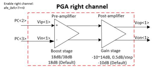
Figure 12-1 Block diagram of PGA
