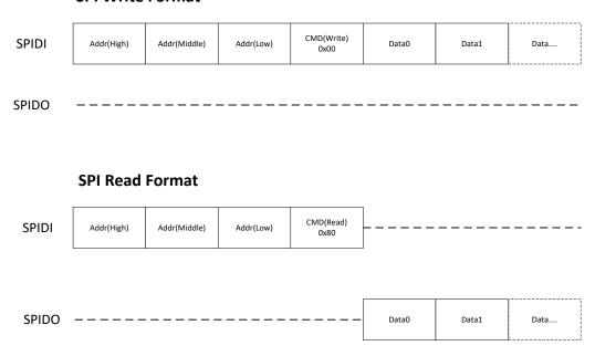
Figure 7-9 SPI write/read command format
