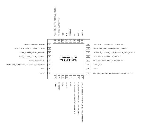
Figure 1-5 Pin assignment for TLSR8258F512ET32/TLSR8258F1KET32/TLSR8258F1KAT32
