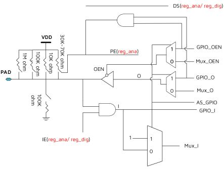
Figure 7-1 GPIO logic diagram
