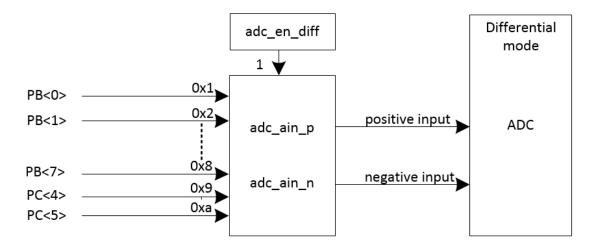
Figure 11-1 Block diagram of ADC
