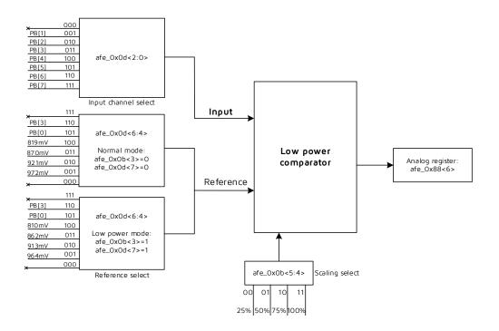
Figure 13-1 Block diagram of low power comparator
