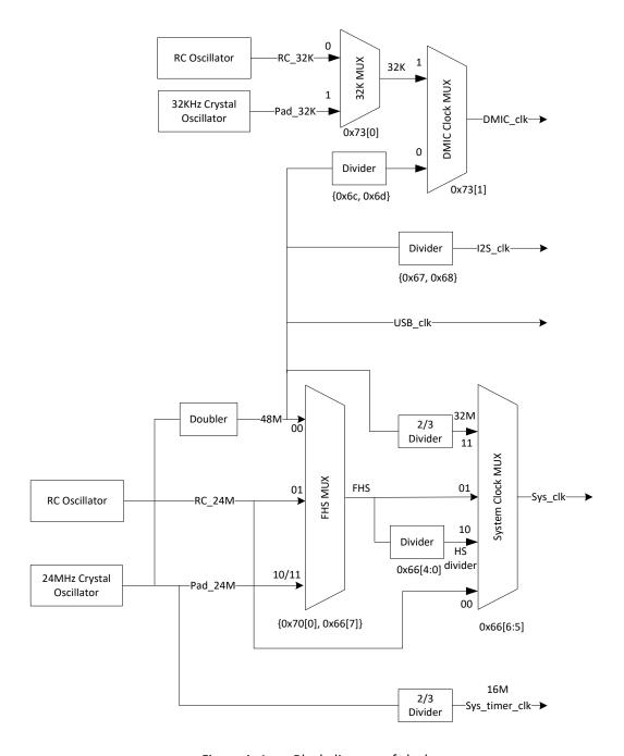
Figure 4-1 Block diagram of clock
