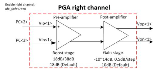
Figure 12- 1 Block diagram of PGA
