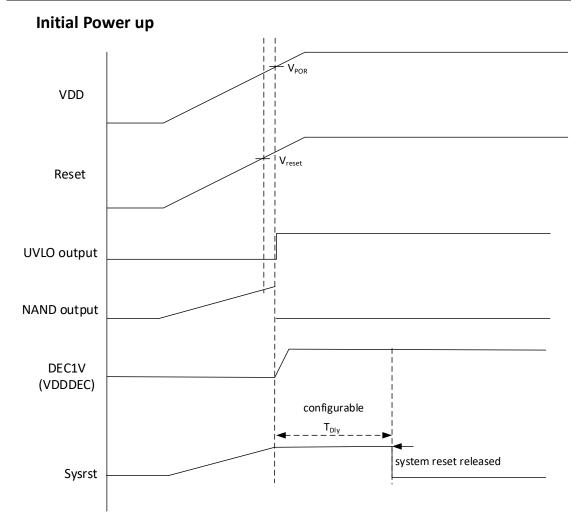
Figure 2-4 Initial Power-up sequence
