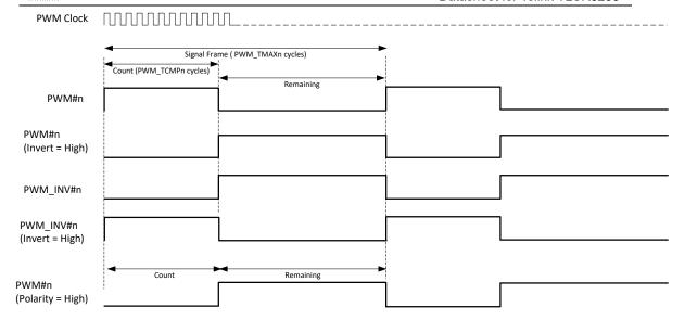
Figure 8-2 PWM output waveform chart
