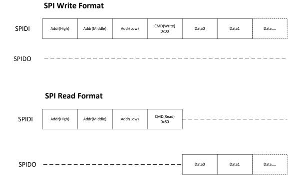
Figure 7-9 SPI write/read command format
