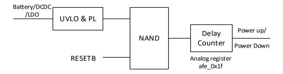
Figure 2-3 Control logic for power up/down
