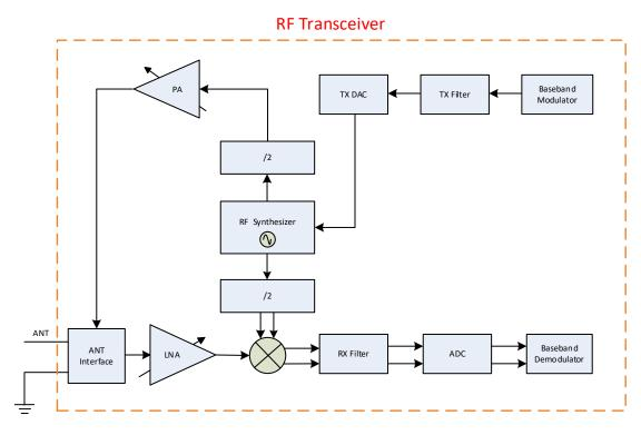
Figure 3-1 Block diagram of RF transceiver
